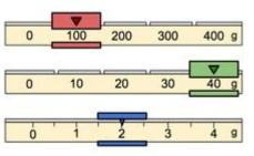
To work a triple beam balance, begin by moving the heaviest weight.
